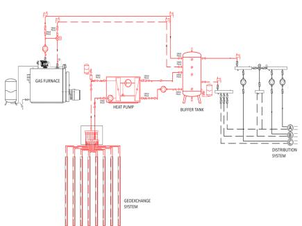
Choosing the right bivalent air temperature point and type of hybrid system is most suitable for retrofit projects in older buildings where a distribution system (radiators or fancoils) and gas furnace is kept (black lines on Figure) and a hybrid system with a heat pump is employed inside the existing engineering (red lines room Figure).
